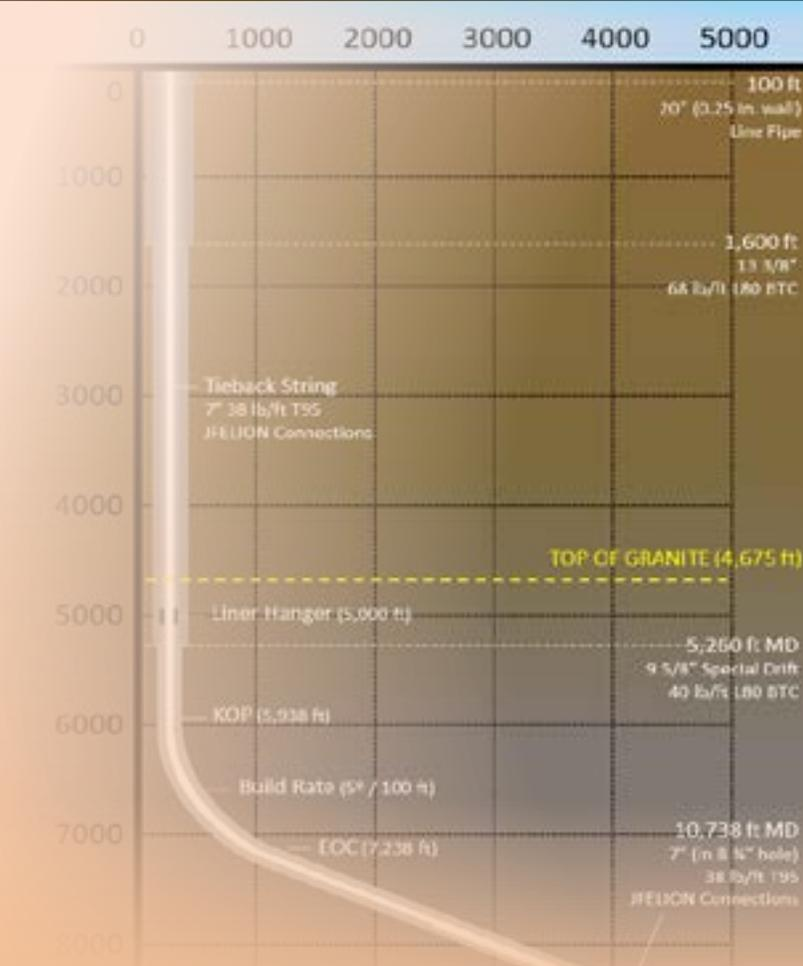
days, including testing, logging, and coring. Most of the hole will be cased with steel pipe that is cemented in place, and only a short interval at the toe will be open (Fig. 2).
