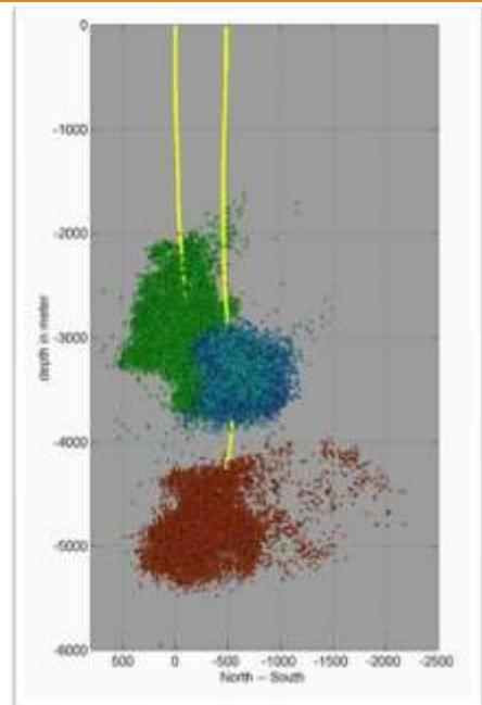
Microseismic cloud induced by stimulation of borehole GPK2 at Soultz-sous-Forets Majer et al 2007
