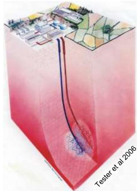
EGS is a concept that first emerged in the early 1970s, having been developed by scientists and engineers working at Los Alamos National Lab, and the graphic captures the essential elements.
