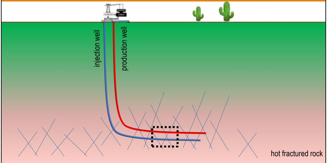
This is a cross sectional view or vertical slice extending to a few kilometres depth showing the subsurface setting of an EGS Hot Dry Rock reservoir.
