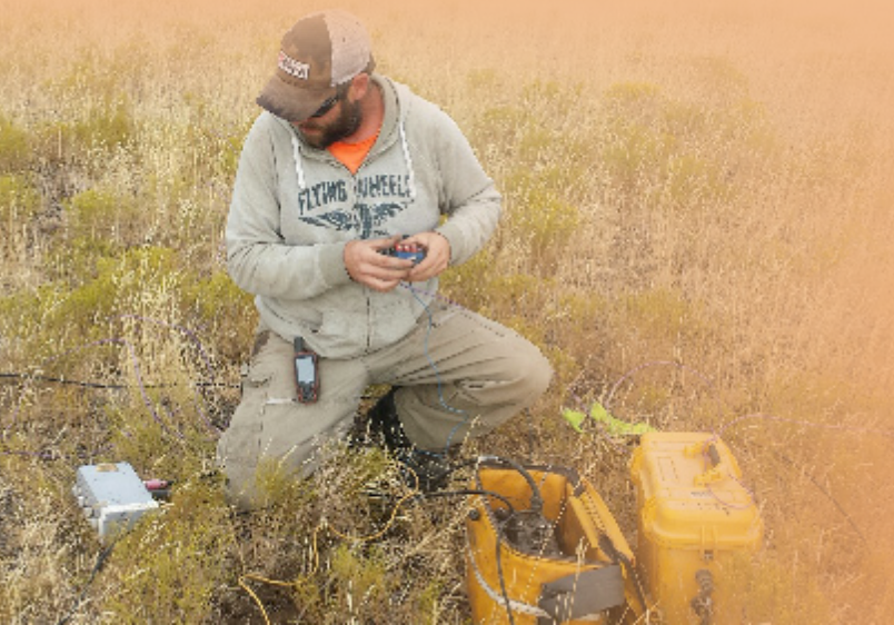
Figure 1. Layout of MT site center near the Utah FORGE project area by contractor Quantec Geoscience. Recorder digitizer is in orange soft-side case, battery pack in yellow hardened case, and magnetic field coil junction as grey metal box.
